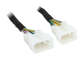
This harness will allow the factory amplifier to be bypassed without altering the factory wiring. Wires are 20 gauge, and 12 inches in length
