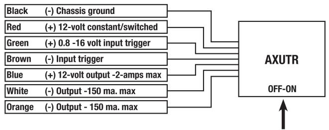
**Programming switch must be turned off after the AXUTR is programmed!**
