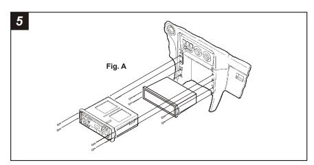
ACCENT: Re-connect the battery terminal and test the unit for proper operation. Mount the head unit/kit assembly to the sub-dash with (4) Phillips screws previously removed in step #1. ELANTRA. TIBURON: Re-connect the battery terminal and test the unit for proper operation. Mount the head unit/kit assembly to the sub-dash with (4) #10 x 3/4" Phillips Truss-head Screws supplied.
