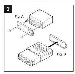
2-SHAFT HEAD UNITS: Slide the aftermarket head unit into the Radio Housing and secure with shaft nuts. (see Fig. A).
