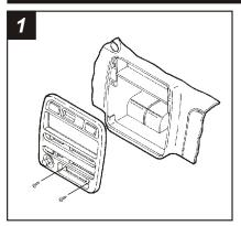
Disconnect the negative battery terminal to prevent an accidental short circuit. For 2002-05 models Remove (2) Phillips screws inside cupholders. Remove the ashtray and (2) Phillips screws exposed.
