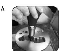
3 Remove the retaining clip at base of shift knob and pull up to remove.
