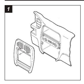
Disconnect the negative battery terminal to prevent an accidental short circuit. Remove (1) screw above the climate controls. Unclip the radio trim bezel and remove. Remove (4) Phillips screws securing the factory radio housing and remove the housing. Disconnect the wiring. Remove (8) Phillips screws securing the factory radio to the factory radio housing and remove the radio. Skip to the Installation Instructions for ALL VEHICLES on Page #2.
