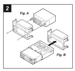
**2-SHAFT HEAD UNITS:** Slide the aftermarket head unit into the **Radio Housing** and secure with shaft nuts. (see Fig. A)
