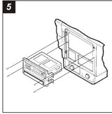
Re-connect the battery terminal and test the unit for proper operation. Mount the head unit/kit assembly to the sub-dash with (4) Phillips screws previously removed in step #1.
