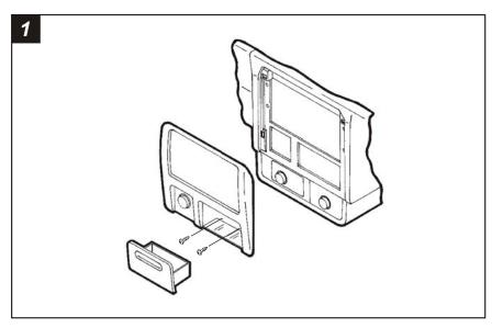
Disconnect the negative battery terminal to prevent an accidental short circuit. Remove the ashtray and (2) Phillips screws exposed in the ashtray cavity. Unclip the radio trim bezel and remove. Remove (4) Phillips screws securing the factory head unit and disconnect the wiring.
