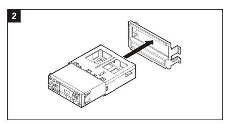
**<u>DIN HEAD UNITS:</u>** Slide the DIN cage into the **Radio Housing** and secure by bending the metal locking tabs down. Slide the aftermarket head unit into the cage until secure. (For a 2-shaft head unit installation, order Metra's **87-09-9902** and snap it into the Radio Housing).
