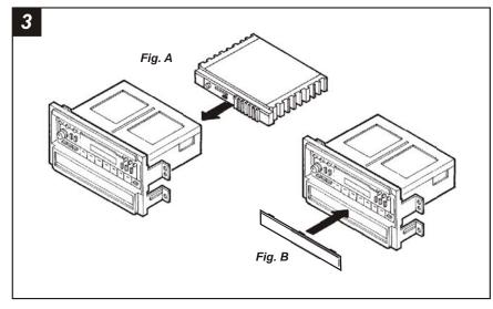
**IF AN EQUALIZER WILL BE INCLUDED:** Slide the aftermarket equalizer into the back of the **Radio Housing.** Using the hardware included with the equalizer, mount the unit to the kit. (see Fig. A)
