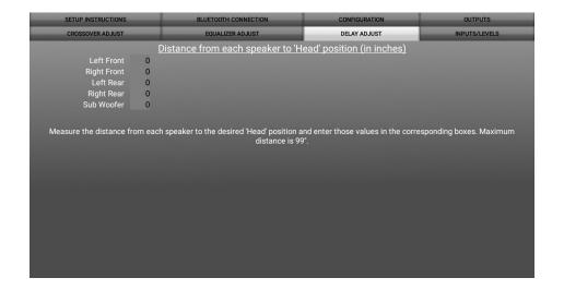
Allows a delay of each channel. If a delay is desired, first measure the distance (in inches) from each speaker to the listening position, then enter those values to the corresponding speaker. Add (in inches) to the desired speaker to delay it.
