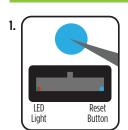
If the interface fails to function, press and release the reset button, then repeat the programming process from step 4 to try again.
