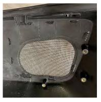
2. Place bag lid on flat surface, covered to protect the Vivid Black painted surface. Working from the inside (Locking latch) to the inside, reinsert the locking mechanism. Insert the latch, and reinstall (4) fasteners into lid and (1) into latch.
