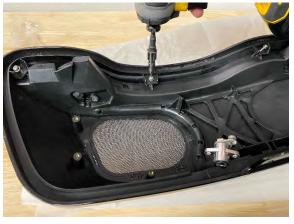
3. Install bag lid strap using (2) T1 coarse threaded fasteners from the original limiting strap, to the locking mechanism.
