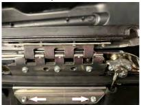
7. Remove the two T15 fasteners for lock (Figure A), and three remaining T15 fasteners (Figure B) on the hinge (Figure C) to the mounting plate (Figure D).
