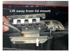
6. Using a T20 bit, remove the two fasteners on the top of the lid.
