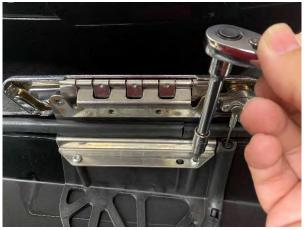
2. Install factory mounting plate, and key lock using T15 machine screws. Then secure remainder of the weather stripping to the hinge plate.
