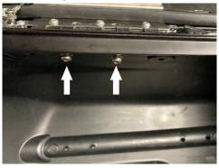
5. Using the razor blade, cut away 2-sided mounting tape away from the lid mount.
