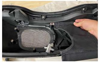
4. Speaker mounting adapters have a LEFT and RIGHT, select the correct adapter and mount to the lid using the (3) Philips fasteners provided. Reusing one factory Torx fastener to the locking mechanism.
