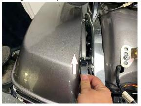
2. Locate quick disconnects on inner of the bag, and rotate counter-clockwise to twist out disconnecting bag from the bike.
