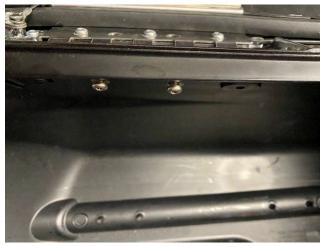
5. Attach the limiting strap to the outer holes, reusing the factory fasteners.
