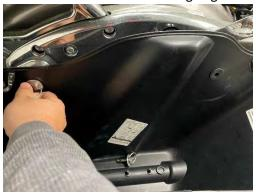
3. Remove bag, and place it on a flat surface. We recommend using a cloth to protect the painted surfaces. Using a T15 wrench, remove the 2 fasteners on the lid strap (Figure A) and the two fasteners from the lid (Figure B).
