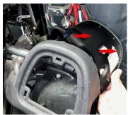
Remove the (2) 11MM bolts from the clamp, securing housing to the crash bar.
