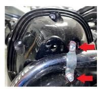
4. Using gentle pressure, push the hosing to the rear of the motorcycle. Remove (3) three, 11mm bolts from the guard.
