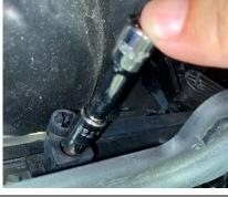
6. Remove slip in the outside, lower corner of the pod to the fairing. Transfer plastic clip to speaker pod.
