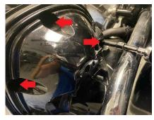
Locate vent level, using a T25 remove bolt and lever from assembly.
