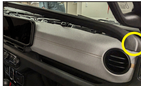
Figure D: With the top trim removed, remove the (2) Phillips screws at the base of the passenger A-pillar.
