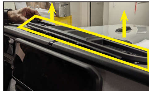
Figure B: Remove the top trim piece with the panel tool.
