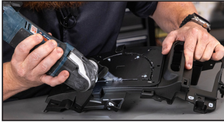
Figure C: Using a cutting tool, follow the channel in the template and cut the dash panel.
