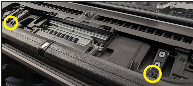
Figure C: With the tray removed, remove the (2) exposed Phillips screws.
