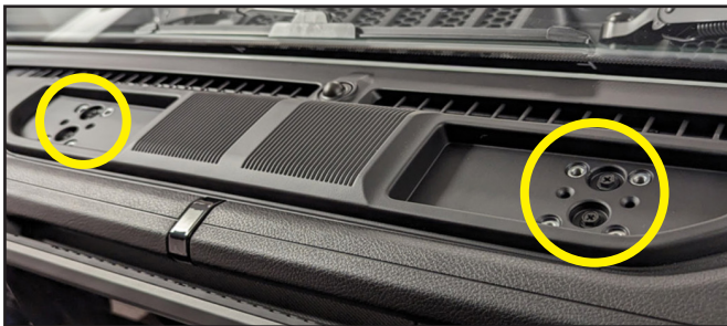
Figure A: Remove (4) Phillips screws from the tray above the radio.
