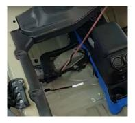
8. Mount the black ground wire to the factory ground points in the kick panels with a 10 mm socket. Scrape paint away from ground mounting location to expose bare metal. The ground wires ring terminal must be placed against the metal of the vehicle. Run ground wire to under seats.
