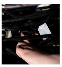
3. Pull back carpet and locate the floor grommet under the seats. Remove grommets. Using a ½ inch drill bit, drill hole in each grommet.
