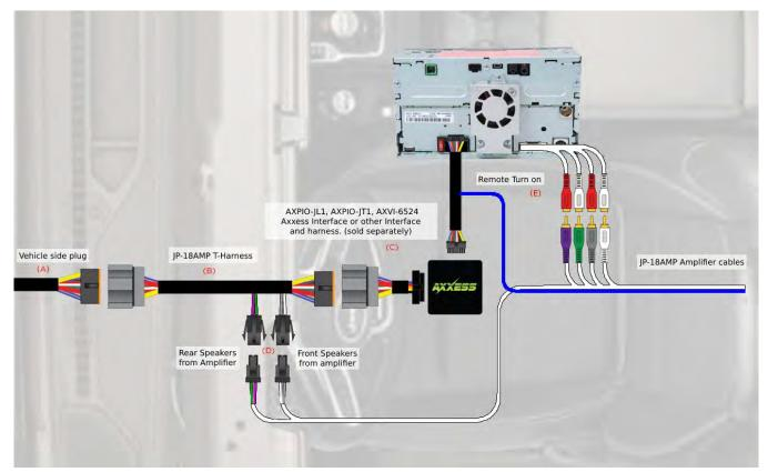
14. Connect the four channels of RCA directly into the RCA outputs of the aftermarket radio, (front left, front right, rear left, rear right). Connect the subwoofer RCA to the sub output of the aftermarket radio, and connect the remote turn on wires to the remote of the aftermarket radio. (**E**)
