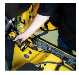
9. Using a pull rod, route the RCA and remote wire cable from the radio cavity then under the center console, the 4-channel cabling goes to the drivers side, the Subwoofer route to the passengers side.
