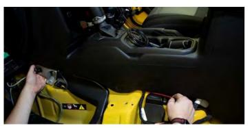
10. Route subwoofer wire under trim until you reach the rear bench seat. Then pull up carpet, and route wires under carpet into the cargo area and connect to subwoofer box. Use caution to avoid the scissor mechanism used to fold the seat down.
