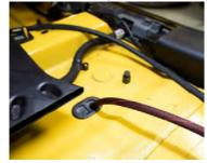
7. Run white power wire across engine bay from vehicle specific fuse holder, following the firewall across, going over the brake booster and down the firewall. Follow the Jeeps frame watching for pinch points, or exhaust components to drivers grommet floor hole. Secure wire with included zip ties. Slide grommet over white power wire and install grommet.
