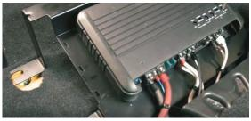
12. Terminate cables with proper connector for the style of amplifier being used. Connect cables and RCAs to the amp. We recommend using InstallBay PN: IBLUGT, and IBFCRIMPER to terminate the ferrules.
