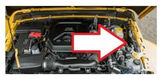
3. Slide Red and Gray tab into locking position pushing forward, route and securing the JP-LAH1 harness. We recommend 4" zip ties. (Metra PN: IBR82)
