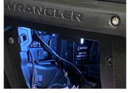
5. Using panel removal tool, remove the Start/HVAC panel
