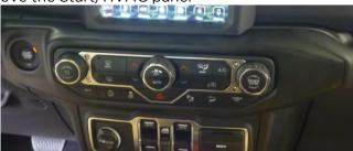
6. Remove (1) screw holding the accessory panel to the sub-dash. Locate panel clips and carefully pull each section free; this may require the panel removal tool.
