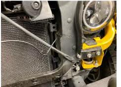
20. Connect the "Grille Tubes Lights" to the cable routed into radiator area. 10" tube can be secured by zip tie (as shown) or clamp.
