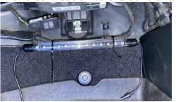
10. Take Passenger interior harness, connect to dash tube and route wire under door sill trim, carpet, and under the passengers seat. Connect harness to under seat tube and secure to seat.
