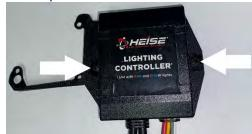
4. Using a T-20 locate and remove the two OE screws, and mount the controller bracket.
