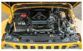
18. Starting at one side of the grille, firmly pull out on the bottom edge to release it from the panel. Continue this process across the entire lower edge until grille is free.
