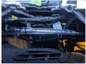
12. Using a semi-rigid wire fishing tool, insert the wire tool in the cavity of the center console just in front of the carpet snap. Fish the cable from the driver side tube across the center console to the passenger side.
