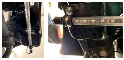
22. Route cable to passengers side (right) front wheel well and mount rock light using the supplied hardware, carefully drill 3/8" hole to pass connector through. Secure rock light to fender well
