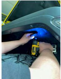
23. Continue to pull cable to passengers side (right) rocker, using the supplied hardware clips and self-tapping screws.
