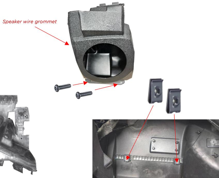
13. Place sub enclosure into footwell area, with the (3) captured nuts facing up. Pull enclosure up from inside dash cavity, secure using M6x12 screws around roll bar.
