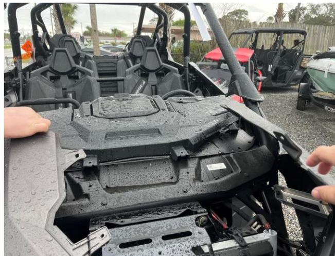
9. Gently pull up on the fenders to remove the locating clips, repeat with the other fender.
