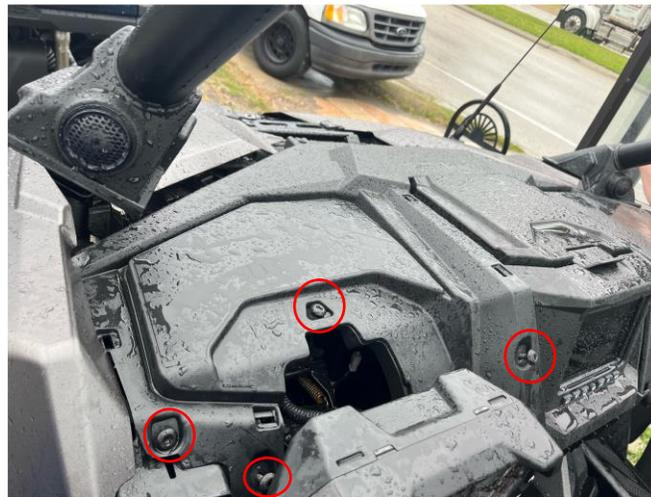
9. From the passengers side, remove the (7) T-20 TORX bolts remaining bolts. *NOTE: The glovebox is lost with installation of sub-enclosure*
