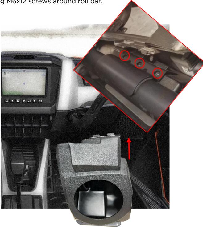
14. Holding the bottom of the enclosure tight to the firewall, line up speed nuts with enclosure holes. Install two included Torx bolts into speed nuts.
