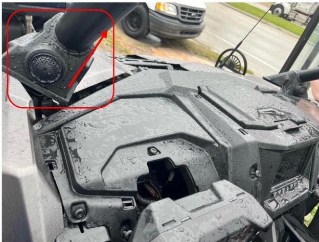
6. Remove (4) T-40 bolts from dash panel on the drivers side of the vehicle.
