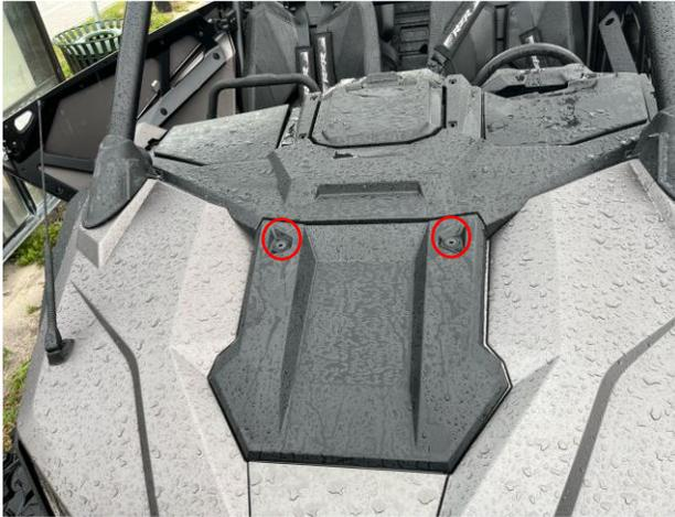
2. Remove two (2) T-40 TORX bolts located under hood holding dash in place.
